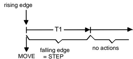
A rising edge at the input sends a MOVE and time T1 (slat adjusting time) is started. If a falling edge is detected within T 1, the binary input sends a STEP. This function is used for the adjustment of the slats. T1 should correspond to the time needed for a slat rotation through 180°.
