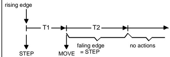
A rising edge sends a STEP and time T1 (time between short- and MOVE operation) is started. This STEP serves the purpose of stopping a continuous run. If a falling edge is detected within T 1, the binary input sends no further telegram.
