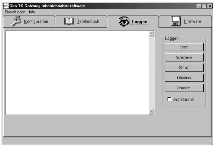
With the "Loggen" ("Logging") function, activities of the commissioning software and the TC-gateway can be logged. Logging helps locate any faults in the communication of the TC-gateway with the Gira door communication bus.
