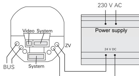
**⚠ When an additional power supply is connected, remove the bus coupler jumpers**
