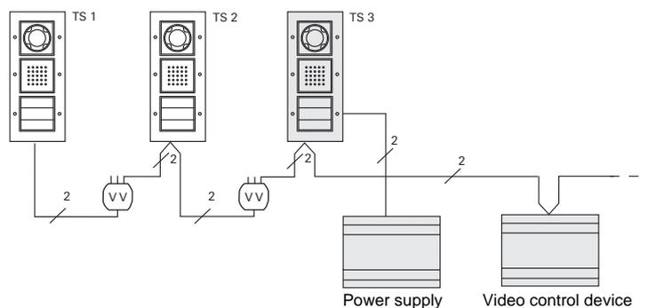
**⚠ When an additional power supply is connected, remove the bus coupler jumpers**
