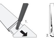
Carefully detach the circuit board from the lower housing section using the appropriate tools. Ensure that the locking hook (see arrow) is pressed next to the screw hole. Do not remove the protective foil from the batteries!
