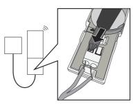
7. Place the upper housing section on the lower section and screw it into place.
