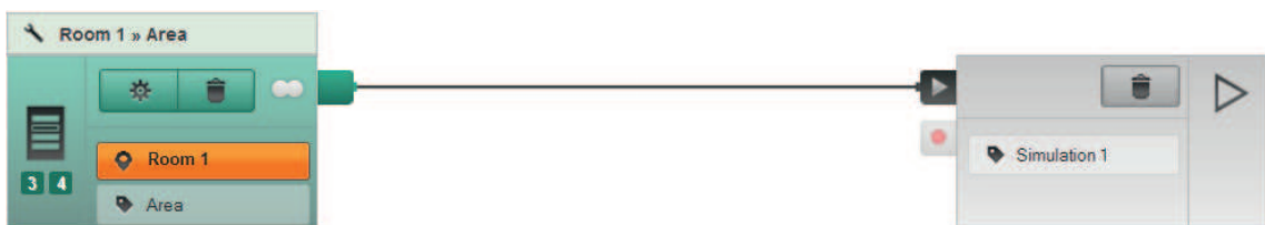
Figure 38: Sensor channel with simulation module for the playback of a simulation
